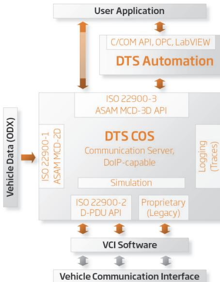
**Figure 1: System Overview of Diagnostic Runtime System DTS COS and DTS Automation**
