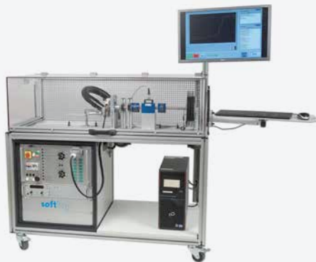
▲ Fig.: Component test bench for power-window motors
