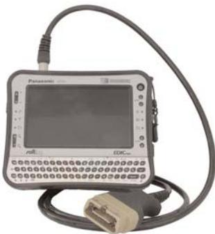
interfaces K-line, CAN and LAN. Due to its dimensions (approx. 184mm x 151mm x 57mm) and the HSDPA module available as an option, the EDICmpc is particularly suitable for use on the road.
