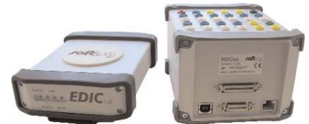
EDICfab is perfect for use in Service and Manufacturing thanks to its ruggedized aluminum profile housing, the shock-absorbing protective caps and connectors in accordance with IP54. The implementation of a modern 32-bit CPU (PowerPC 384 MHz) has resulted in a high-performance platform for powerful diagnostic and flash applications.
