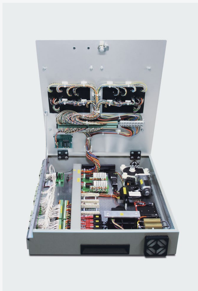
▲ Fig.: Test adapter for door control units
