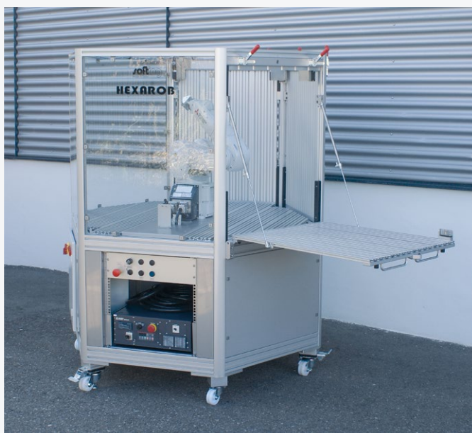
▲ Fig.: Driver simulation through articulated-arm robot
