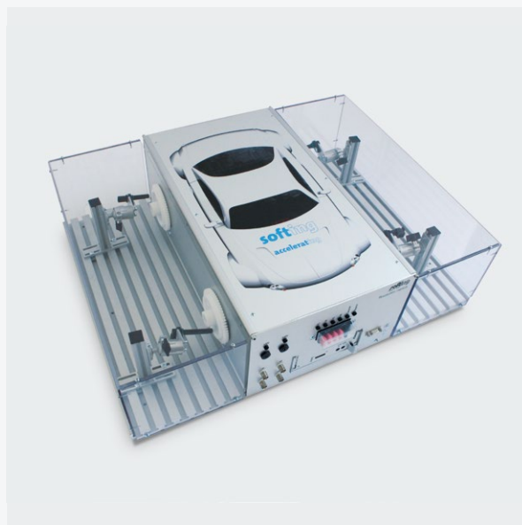
▲ Fig.: Wheel speed simulation
