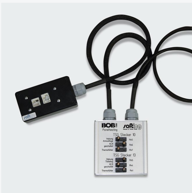
▲ Fig.: Measuring adapter for door control units
