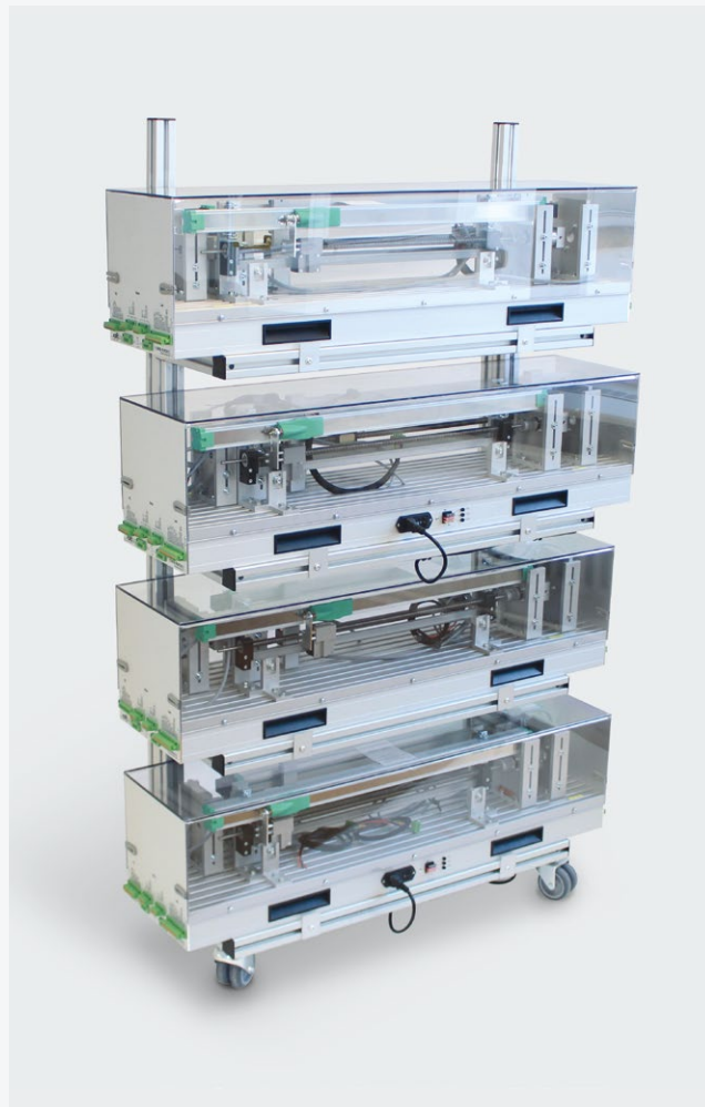
▲ Fig.: Simulation of seat adjusting motors
