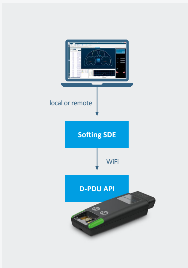
▲ Fig.: Setup of a Typical Diagnostic Tester
