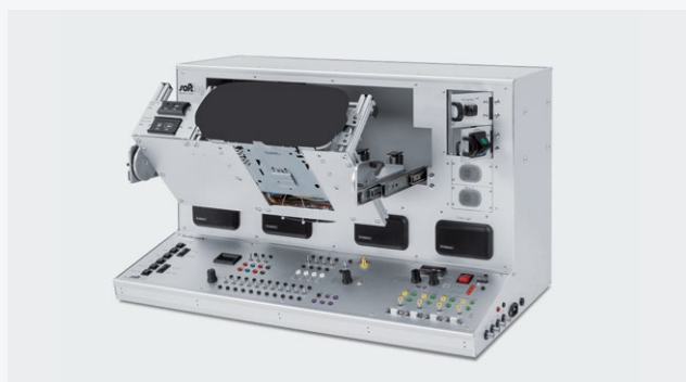
▲ Fig.: Lab car for a radio (HeadUnit)
