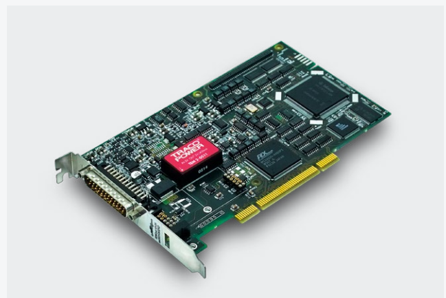
▲ Fig.: EDICpci, High-performance VCI with PCI interface for stationary applications
