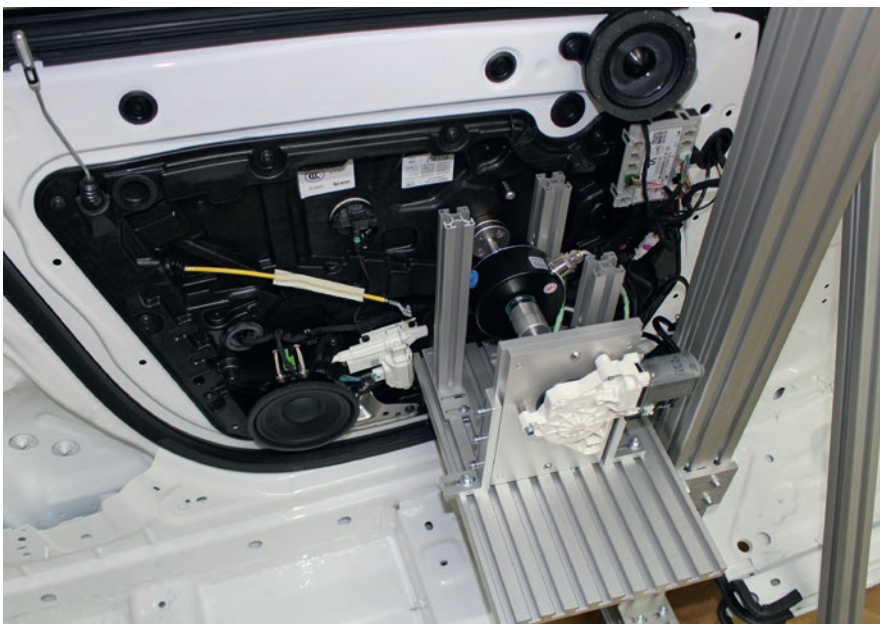
Mechatronic simulation: force measurement and influence on the window regulator
