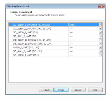
Assign the pins of the HS interface to the appropriate logical connection (see image above).
